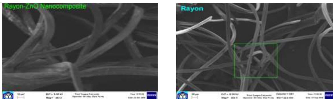
**Figure 5** SEM micrographs of synthesized rayon and rayon-ZnO nanocomposite
