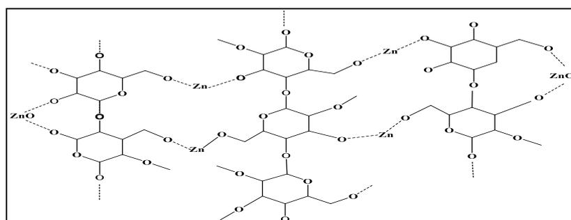
**Figure 4** Proposed structure of synthesized rayon-ZnO nanocomposite
