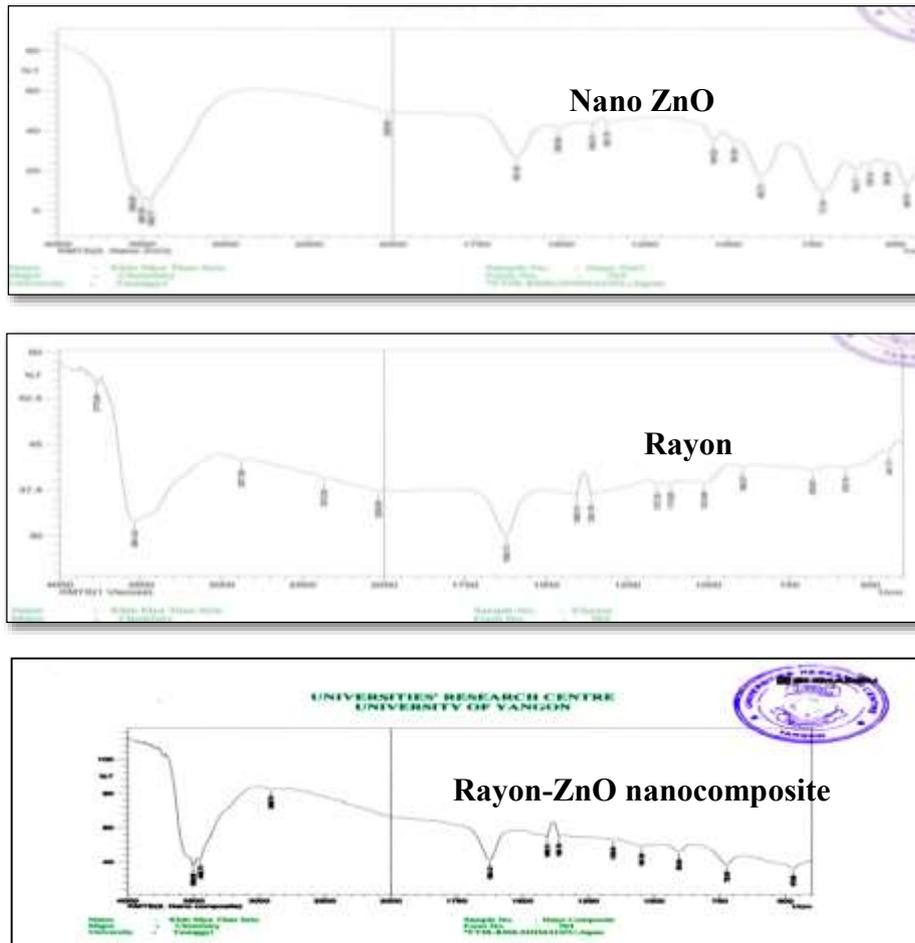
**Figure 3** FT-IR spectrum of synthesized rayon, nano ZnO and rayon-ZnO nanocomposite
